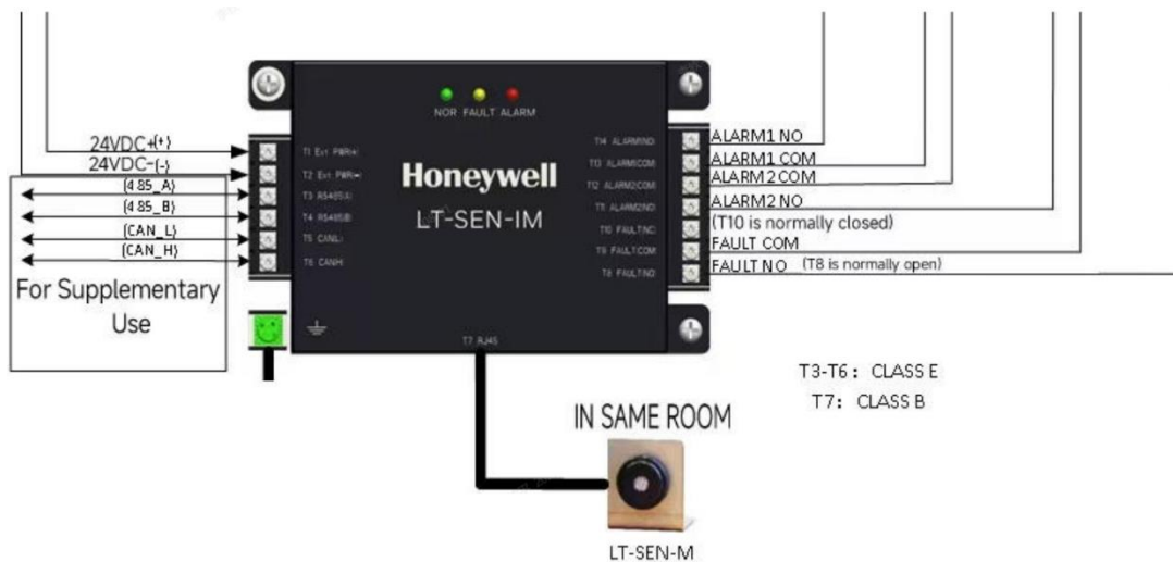
Figure 7-4 Flammable Gas Detector Wiring Diagram
