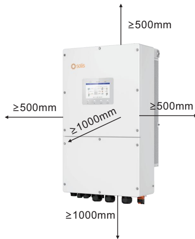
Figure 3.5 Inverter Mounting Clearances
